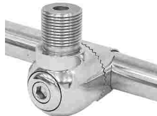
LOW-PROFILE ANTENNA RATCHET MOUNTS casted AISI 316 no handle installation on rails of 7/8"(22mm) and 1"(25mm). ITEM NO. Thread Weight/g 009692 1"~14" 450
