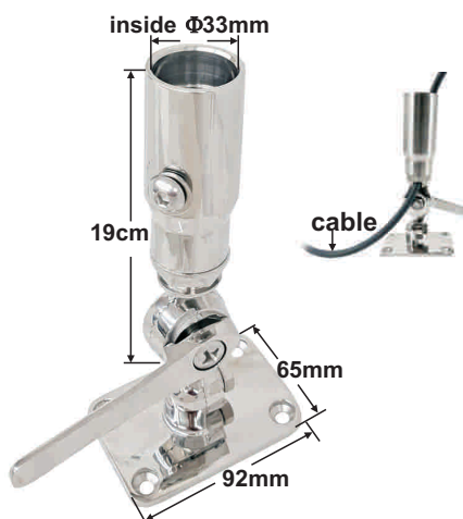
STARLINK ADAPTER AND RATCHET BASE casted AISI 316 Starlink 316 stainless steel adapter to mount to a 1"-14 thread Bottom of the adapter has 1"-14 threads and comes with locking nut Top of the adapter is machined to fit the starlink antenna post The overall height is 19cm (adapter with the ratchet base) Base measures 65mm(2-1/2")x92mm(3-9/16") with 4 holes for 1/4" bolts with 3/8" hole for cable pass through ITEM NO. B24-027
