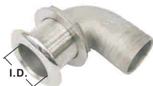
90 DEGREE THRUHULL MUSHROOM HEAD BARBED casted AISI 316 for use with hose, not for use below the waterline ITEM NO. Hose Max Hull Flange size Thickness O.D.mm I.D.mm Weight/g 010007 25mm 29 mm 43 33 183
